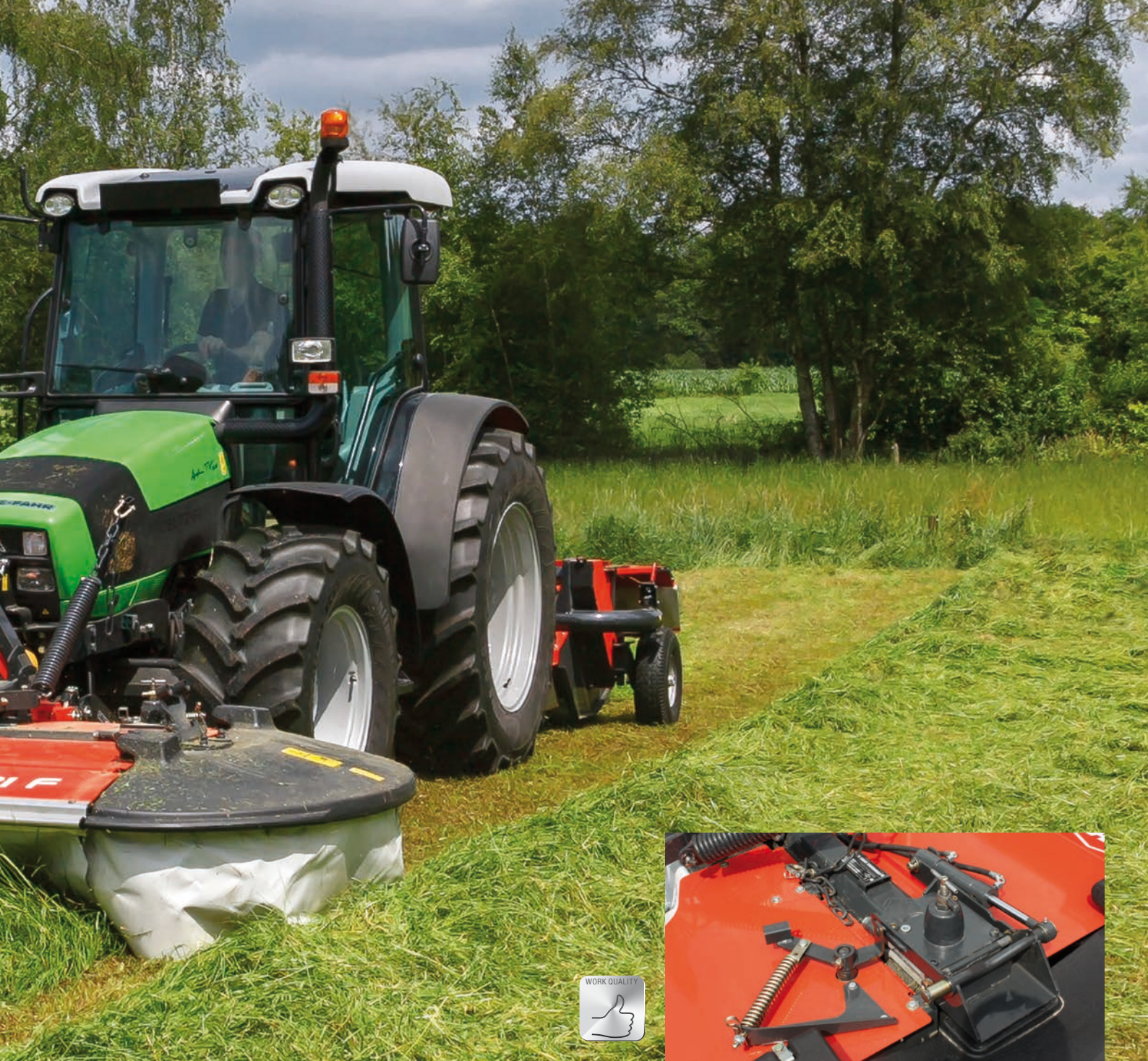
Hydraulic folding device for side covers
