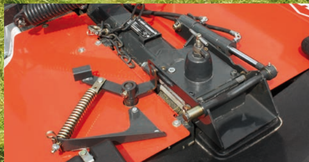
Hydraulic folding device for side covers
