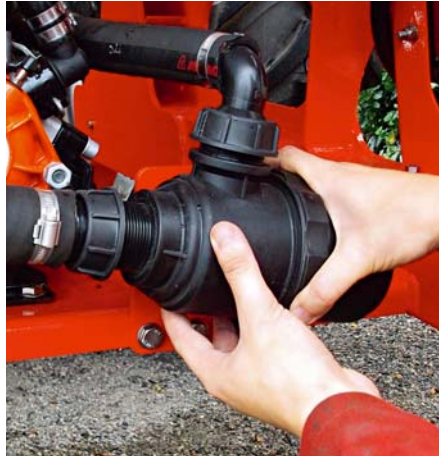
Suction filter on the pump intake.
